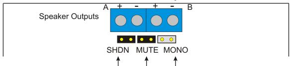
**SHDN** is for external switch to put the amp in Stand-By Mode- jumper On = amp On - Off = Standby **Mute** is to add external Mute Switch - jumper On = Sound - Off = Mute **Mono** is to put the amp in bridge single channel mode - Off = Stereo - On = Bridge Mode
